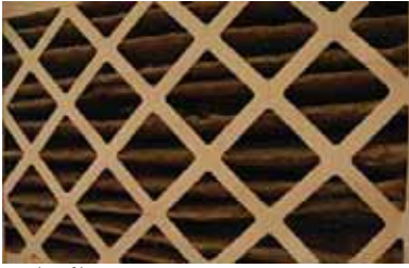
Used air filter. Source: MosArt Architecture.
